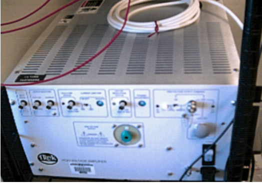
Figure 6 Trek Model PO923A HV Power Amplifier, used for driving the capacitor at 2 kV and 400 mA.
