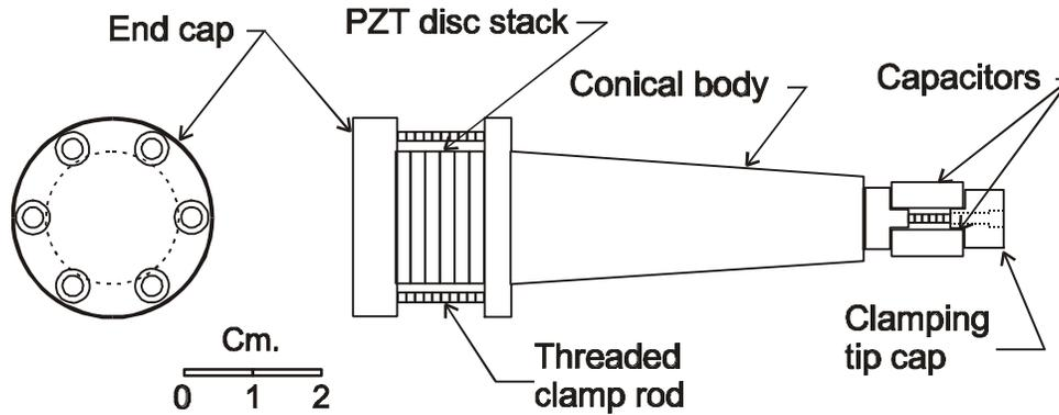
**FIGURE 3.** A third generation device currently under test. The configuration is modeled after that of an ultrasonic transducer in an attempt to maximize the driven excursion of the capacitors at its tip.
