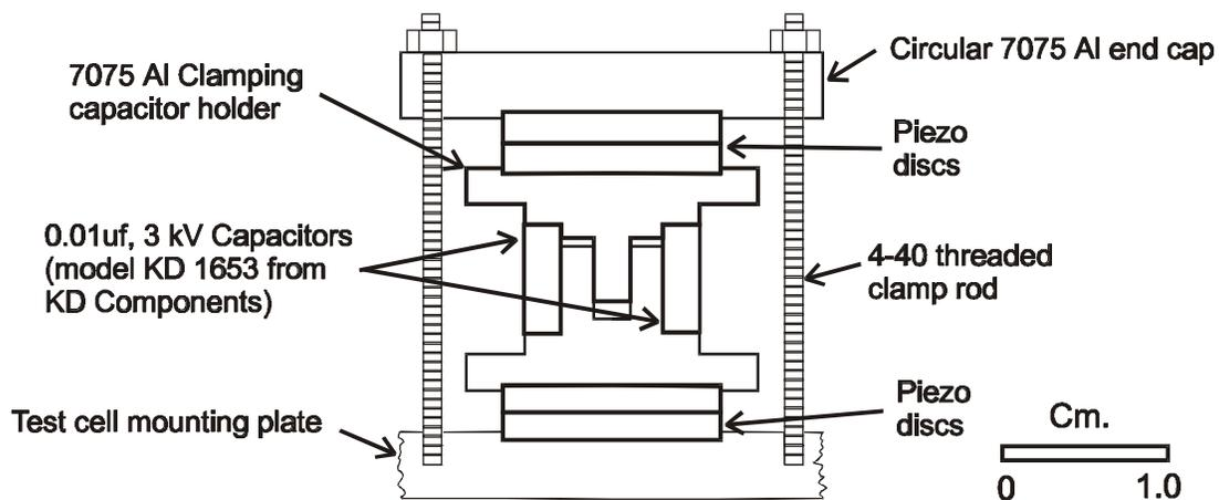
**FIGURE 1.** A scale, cross sectional view of a second generation device. The capacitors are held in an aluminum capacitor holder, which is in turn sandwiched between two PZT stacks.
